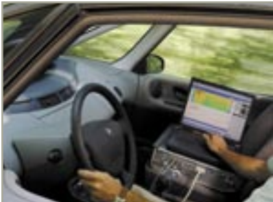
Measure acoustic and acceleration signals on the road or roller bench and calculate on-line metrics related to the human perception of noise.
