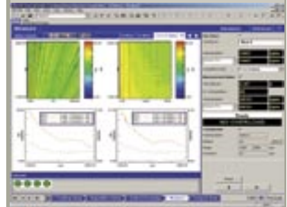
Fixed and synchronous sampling on torsional vibration signals support analysis in the time/frequency or in the angular/order domain.
