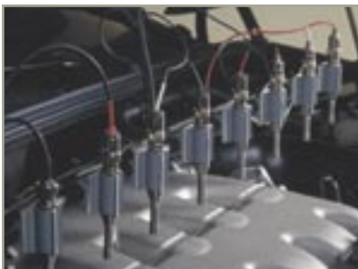
Measure and evaluate the product's acoustic performance with multiple microphones connected to a light and portable acquisition system.
