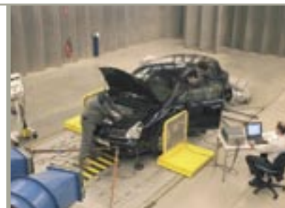
Noise and vibration engineers perform benchmarking, troubleshooting and design verification on test benches or in operating conditions.
