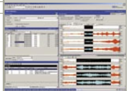
Use the time signal calculator for removing average rpm or to derive shaft torsion.
